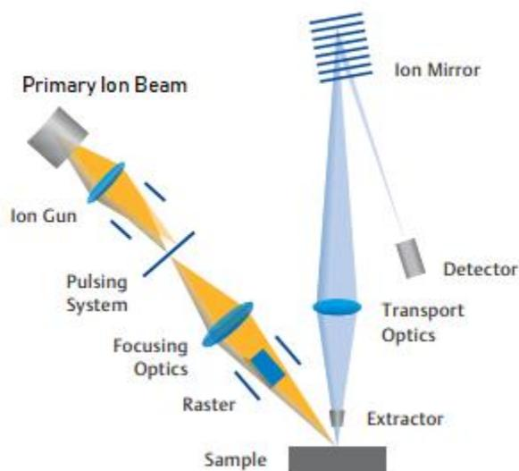
Each point of impact on the sample from the primary ion beam contains the entire mass spectrum, as well as the X, Y and Z coordinates of that point of impact. With this information, we can create detailed ion images of the distribution of any species of interest on our sample, both in 2D and in 3D (in depth profile mode).
